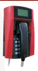
Analogue desk/wall telephone for applications in potentially explosive areas (zones 2 and 22). This telephone comprises a housing made of impact-resistant thermoplastic and is certified according to ATEX. In the field of the chemical and petrochemical industry potentially explosive atmospheres occur during production procedures caused by e.g. gases, vapours or mist.
