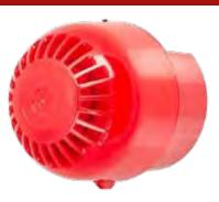
The IS-S-02 Intrinsically Safe Sounder is ATEX and IECEx certified, and is approved to be installed in Groups I (Mining) and Group II (above ground), Zones 0, 1 or 2 with gas groups IIA, IIB, IIC and Zones 20, 21 and 22 for dust groups IIIC and carries a temperature classification of T6.
