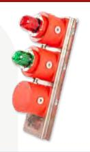
SL 150 combined status lights in GRP. This signalling device is certified for use in ATEX zones 1,2 for gas and 21,22 for dust.
