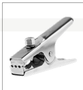
These grounding clamps are especially made for discharging electrostatic charge from potentially endangered system parts. Sharp stainless steel teeth get through insulating layers such as paint, rust, dirt and grease thanks to the high pressure of the spring. In this way an effective "metal-to-metal" connection can be created and a safe grounding guaranteed.
