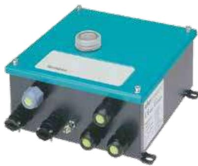
Terrabox TCB030 is designed for direct installation in explosion hazard areas and for connecting a clamp. The dual-color indicator lamp signals the correct grounding state. The integrated contacts allow an enable circuit to be implemented.
