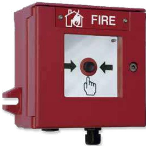
The Ex Manual Call Point is designed for manual fire alert purposes in potentially explosive areas. Its protection type allows for applications in all Ex areas of zones 1, 2, 21 and 22. Type B Manual Call Point according to EN 54-11 or Special Alarm according to EN 12094/EN 12094-1.
