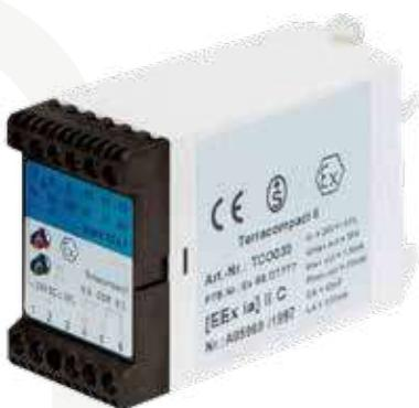
During filling or decanting processes involving solid or liquid materials in the Ex area, the Terracompact II TCO030 automatically identifies faulty or defective ground links in the installation. If the floating changeover contact is switched accordingly, it shuts off the process.
