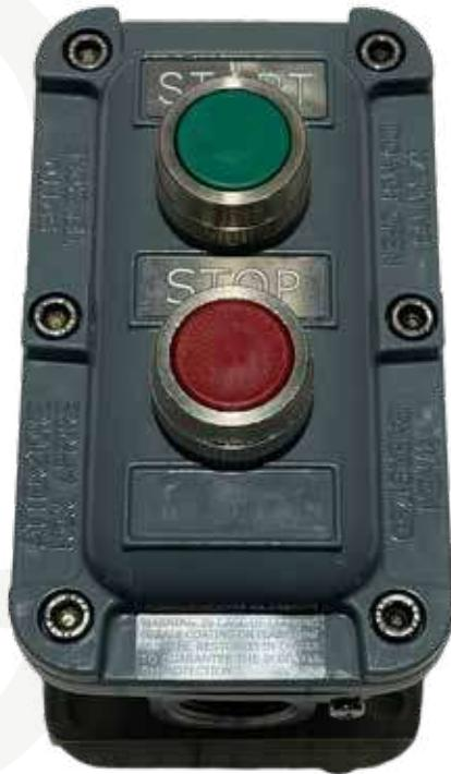
Explosion-proof Start-Stop control panel for use in hazardous areas. Ex d enclosure equipped with a green 2NO pushbutton and a red 2NC pushbutton, fitted with 2 cable entries 3/4" NPT.
