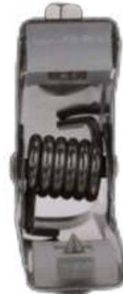
These grounding clamps are especially made for discharging electrostatic charge from potentially endangered system parts. Sharp stainless steel teeth get through insulating layers such as paint, rust, dirt and grease thanks to the high pressure of the spring. In this way an effective "metal-to-metal" connection can be created and a safe grounding guaranteed.
