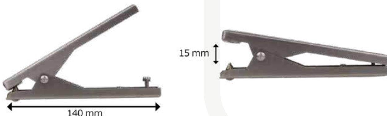
These grounding clamps are especially made for discharging electrostatic charge from potentially endangered system parts. Sharp stainless steel teeth get through insulating layers such as paint, rust, dirt and grease thanks to the high pressure of the spring. In this way an effective "metal-to-metal" connection can be created and a safe grounding guaranteed.
