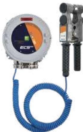
ECS-RF series electronic equipment provides earth connection of process equipment (road tankers, drums, IBCs, etc..) with real-time ground connection monitoring. The system monitors that connection to earth is obtained with a resistance lower than  $10\Omega$ , according to the ATEX Directive 2014/34/EU.
