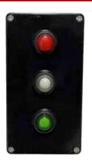
ATEX-certified control panels equipped with 3 pilot lights, made of glass-fibre reinforced polyester for use in explosive atmospheres.
