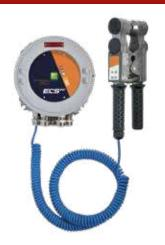
ECS-RF series electronic equipment provides earth connection of process equipment (road tankers, drums, IBCs, etc..) with real-time ground connection monitoring. The system monitors that connection to earth is obtained with a resistance lower than  $10\Omega$ , according to the ATEX Directive 2014/34/EU.
