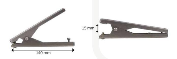
These grounding clamps are especially made for discharging electrostatic charge from potentially endangered system parts. Sharp stainless steel teeth get through insulating layers such as paint, rust, dirt and grease thanks to the high pressure of the spring. In this way an effective "metal-to-metal" connection can be created and a safe grounding guaranteed.
