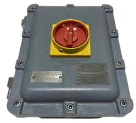
32A, 3-pole ATEX certified load break switch for use in explosive atmospheres. Suitable for classified zones 1, 2, 21 and 22.
