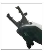
These grounding clamps are especially made for discharging electrostatic charge from potentially endangered system parts. Sharp stainless steel teeth get through insulating layers such as paint, rust, dirt and grease thanks to the high pressure of the spring. In this way an effective "metal-to-metal" connection can be created and a safe grounding guaranteed.
