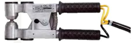
The electrical continuity is ensured by the carbonitrided steel contact tips which make a firm connection to any foothold having a thickness between 3 and 20 mm.
