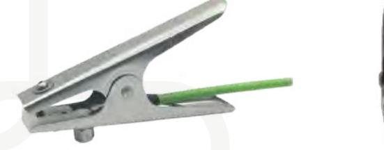
These grounding clamps are especially made for discharging electrostatic charge from potentially endangered system parts. Sharp stainless steel teeth get through insulating layers such as paint, rust, dirt and grease thanks to the high pressure of the spring. In this way an effective "metal-to-metal" connection can be created and a safe grounding guaranteed.
