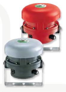
The signalling bell dGW21 was designed to warn, call and signal in areas with explosive atmospheres in group II and rough ambient conditions. The protection type II 2G Ex de IIC T6 allows the signalling bell to be used without restriction in all ex-areas classified 1 and 2.
