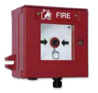
The Ex Manual Call Point is designed for manual fire alert purposes in potentially explosive areas. Its protection type allows for applications in all Ex areas of zones 1, 2, 21 and 22. Type B Manual Call Point according to EN 54-11.
