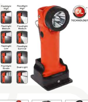
The XPR-5568RX Intrinsically Safe angle light is a flashlight, a floodlight and a Dual-Light angle light that is cULus, ATEX, IECEx and MSHA certified Intrinsically Safe. The flashlight rotates 90 degrees up and down with a 45 degree downward angled floodlight.
