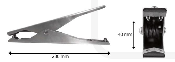
These grounding clamps are especially made for discharging electrostatic charge from potentially endangered system parts. Sharp stainless steel teeth get through insulating layers such as paint, rust, dirt and grease thanks to the high pressure of the spring. In this way an effective "metal-to-metal" connection can be created and a safe grounding guaranteed.
