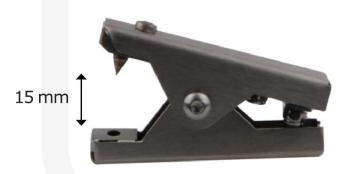
These grounding clamps are especially made for discharging electrostatic charge from potentially endangered system parts. Sharp stainless steel teeth get through insulating layers such as paint, rust, dirt and grease thanks to the high pressure of the spring. In this way an effective "metal-to-metal" connection can be created and a safe grounding guaranteed.
