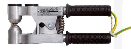
The electrical continuity is ensured by the carbonitrided steel contact tips which make a firm connection to any foothold having a thickness between 3 and 20 mm.
