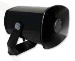
This versatile 25W Ex plastic horn speaker is light in weight and features a spacious connection chamber of protection type 'e'. It has dual M20 entries in the back lid for easy cable mounting and supports loop in loop out as standard.
