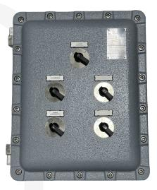
CCF7AG series Ex d enclosure designed to house different types of electrical protections in explosive atmospheres, suitable for use in zones 1, 2, 21 and 22. Each block is operated by means of a robust and reliable non-lockable handle.
